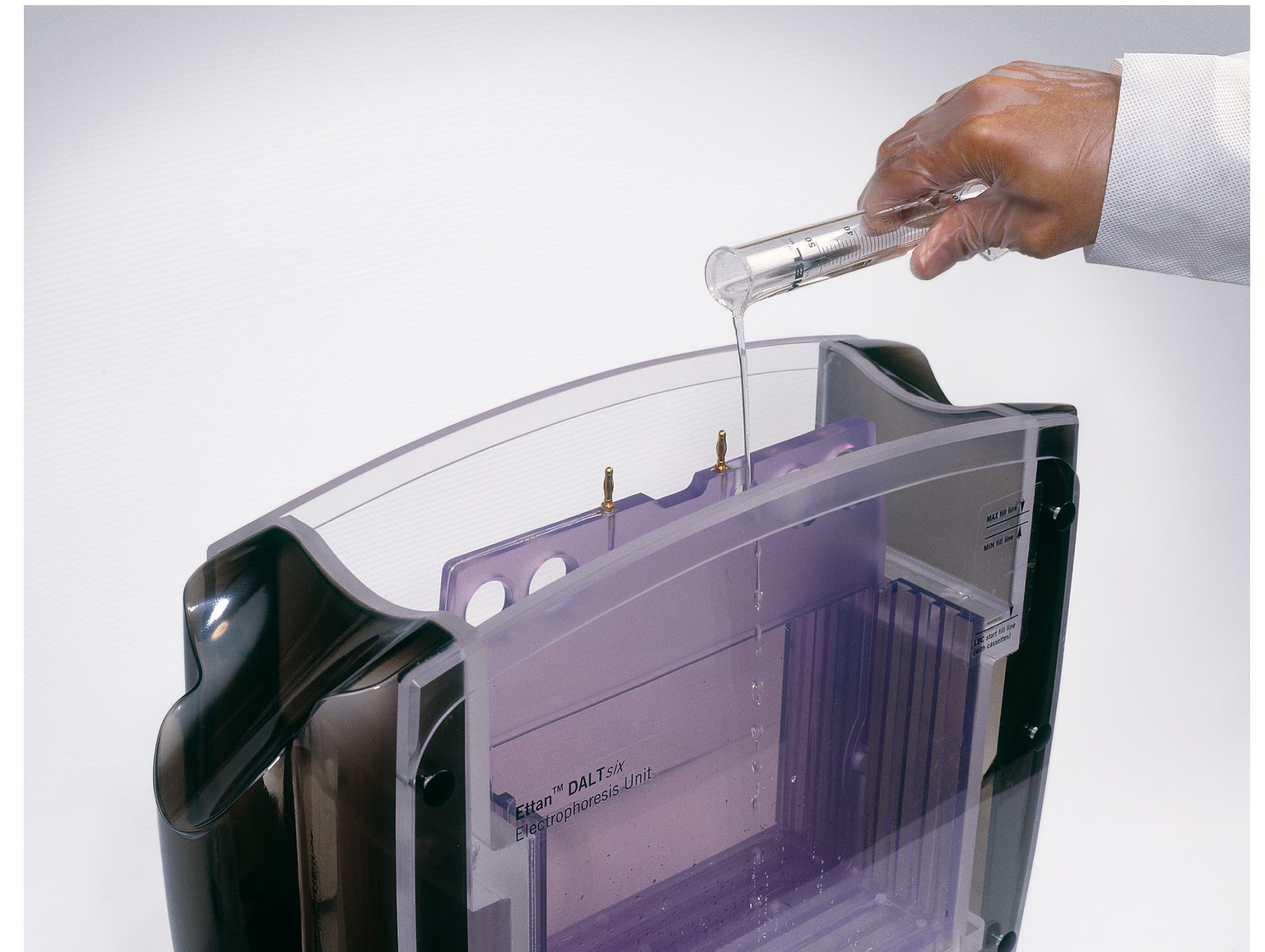
Fig 34. Filling the Ettan DALTsix electrophoresis unit with anode buffer.
